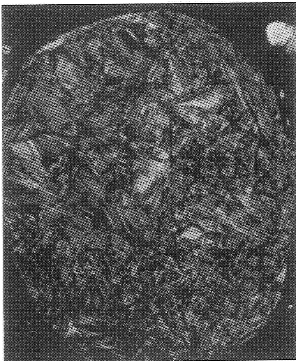
Fig. 3. Optical texture of Cu(LC 16 ) observed with crossed polarizers at 380 K.
